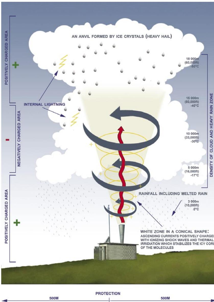
With this gun, every five seconds ionizing (high energy) shock waves go up in the air. These reach very fast the high atmosphere, up to 15000m, at  $-50^{\circ}\text{C}$ , where the hail is created.
